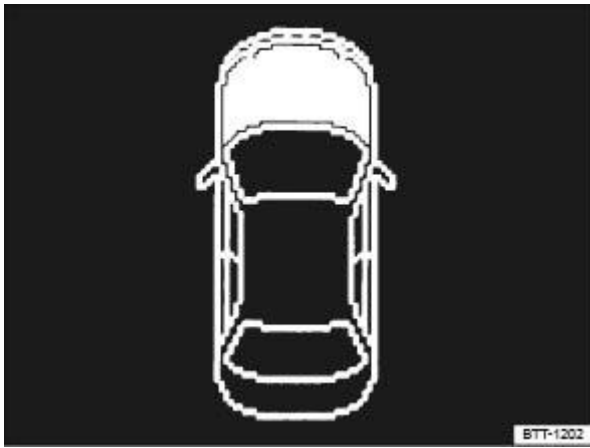
Fig. 184 On the instrument cluster display: the bonnet is open or has not been closed properly.
