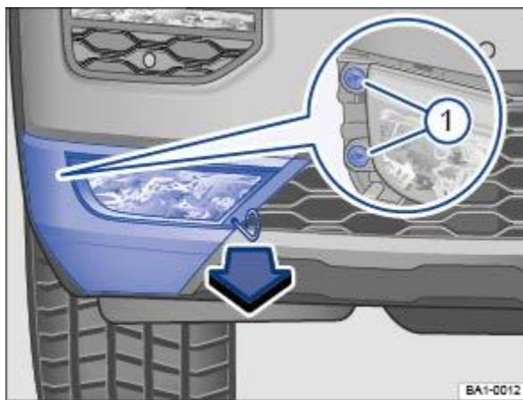
Fig. 169 In the front bumper, right-hand side: removing the fog light.
