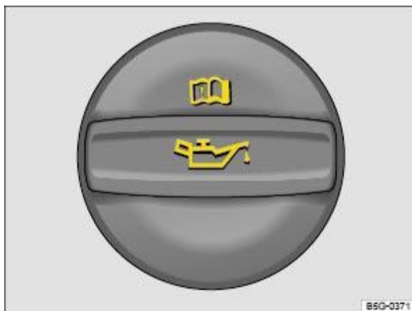
Fig. 187 In the engine compartment: engine oil filler cap (illustration).
