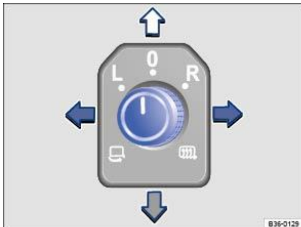
Fig. 88 In the driver door: rotary knob for the exterior mirrors.
