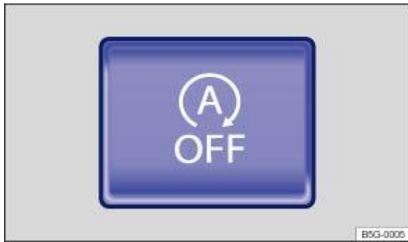
Fig. 102 In the upper part of the centre console: button for the start/stop system.
