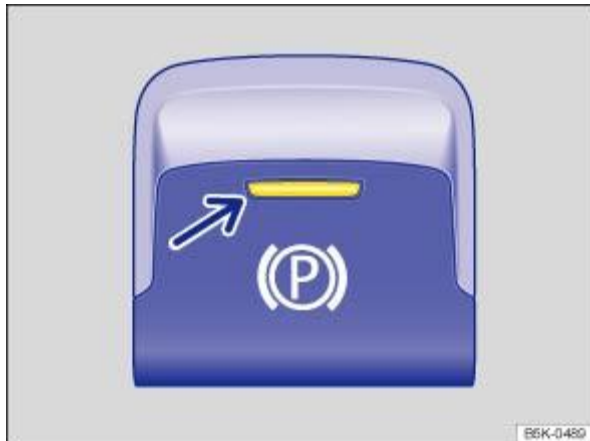
Fig. 125 In centre console: button for the electronic parking brake.
