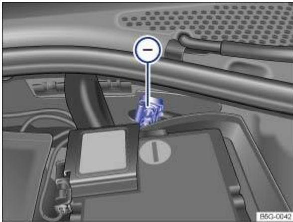
Fig. 176 In the engine compartment: jump lead connection point (earth connection).
