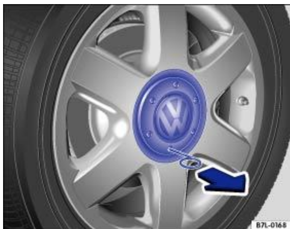
Fig. 199 Removing the centre wheel trim by pulling.
