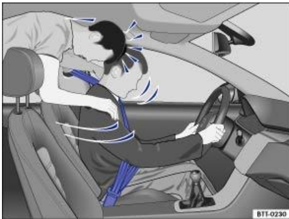
Fig. 32 The unbelted rear passenger is thrown forward and strikes the belted driver.
