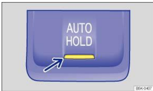
Fig. 126 In the centre console: button for the Auto Hold function.
