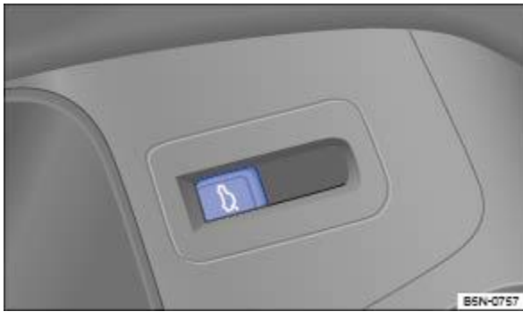
Fig. 61 In the driver door: release button for the boot lid.
