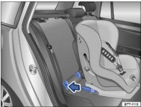
Fig. 47 Illustration: fitting an ISOFIX child seat with attachment arms.
