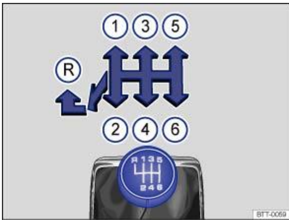
Fig. 104 Gear shift pattern of a 6-speed manual gearbox.
