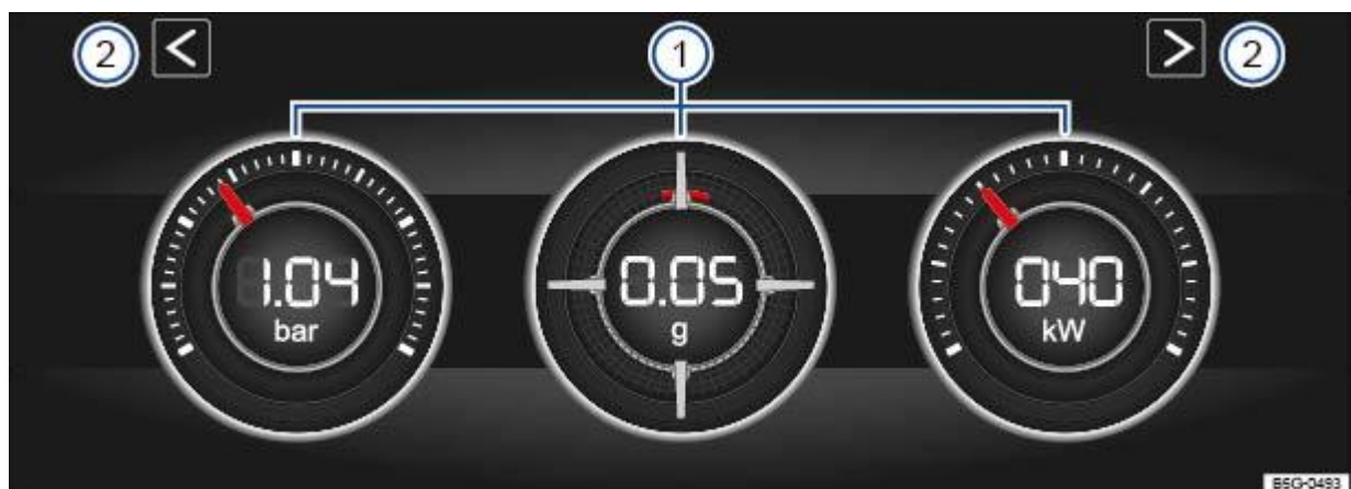
Fig. 23 On the Infotainment system display: performance monitor.
