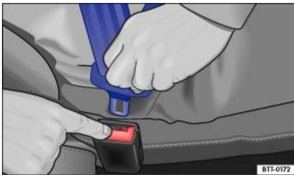
Fig. 35 Removing the latch plate from the buckle.
